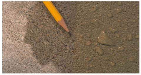
Treating concrete with Dymacryl allows water to bead (right) while untreated concrete (left) is deeply stained by water absorption. Dymacryl prevents water penetration, thereby preserving the appearance of exposed masonry.
